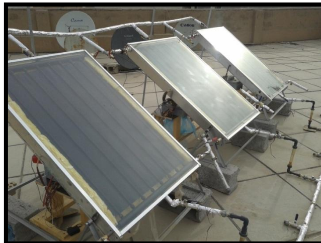
Figure 5. Three flat plate solar collector's connection in parallel mode (Z – Configuration).
