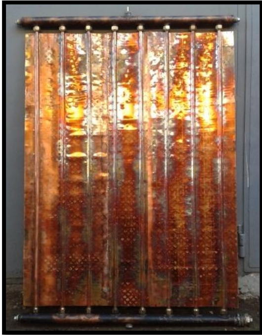
Figure 2. A copper sheet welding on riser pipes.
